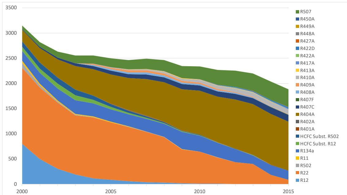
**Figure 9: Emissions of refrigeration installations by refrigerant (kt CO<sub>2</sub>-eq)**
