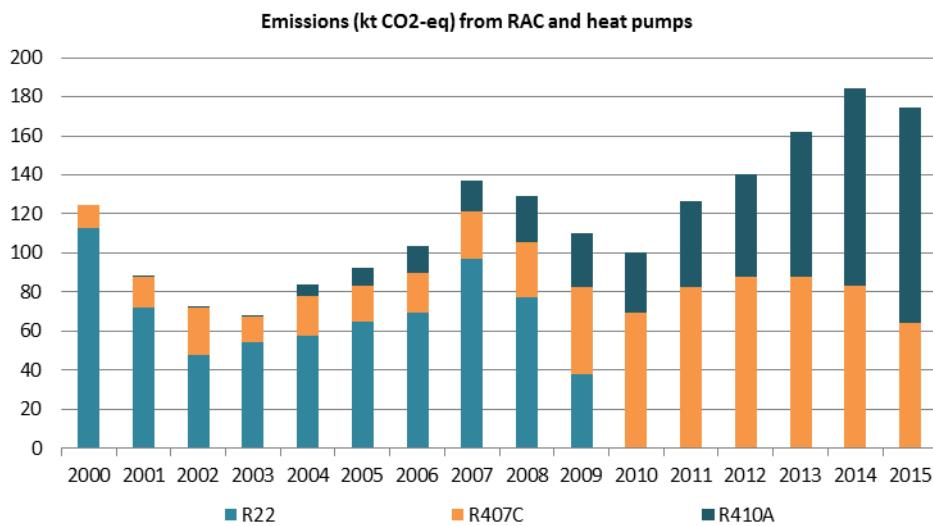
Figure 11: Emissions from room air conditioning and heat pumps (in kt CO<sub>2</sub>-eq)
