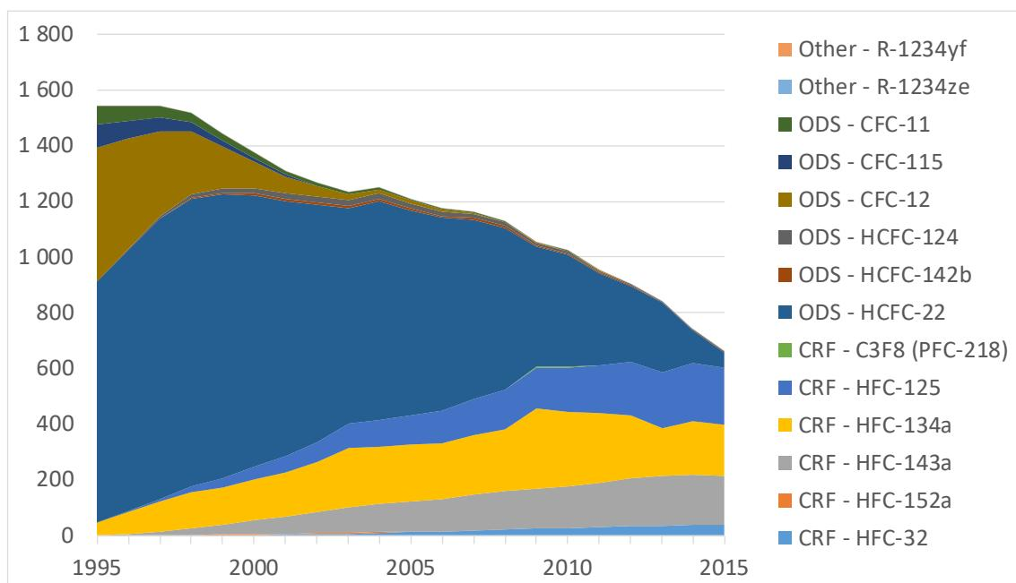
Figure 6: Emissions from refrigeration installations, by substance (t)
