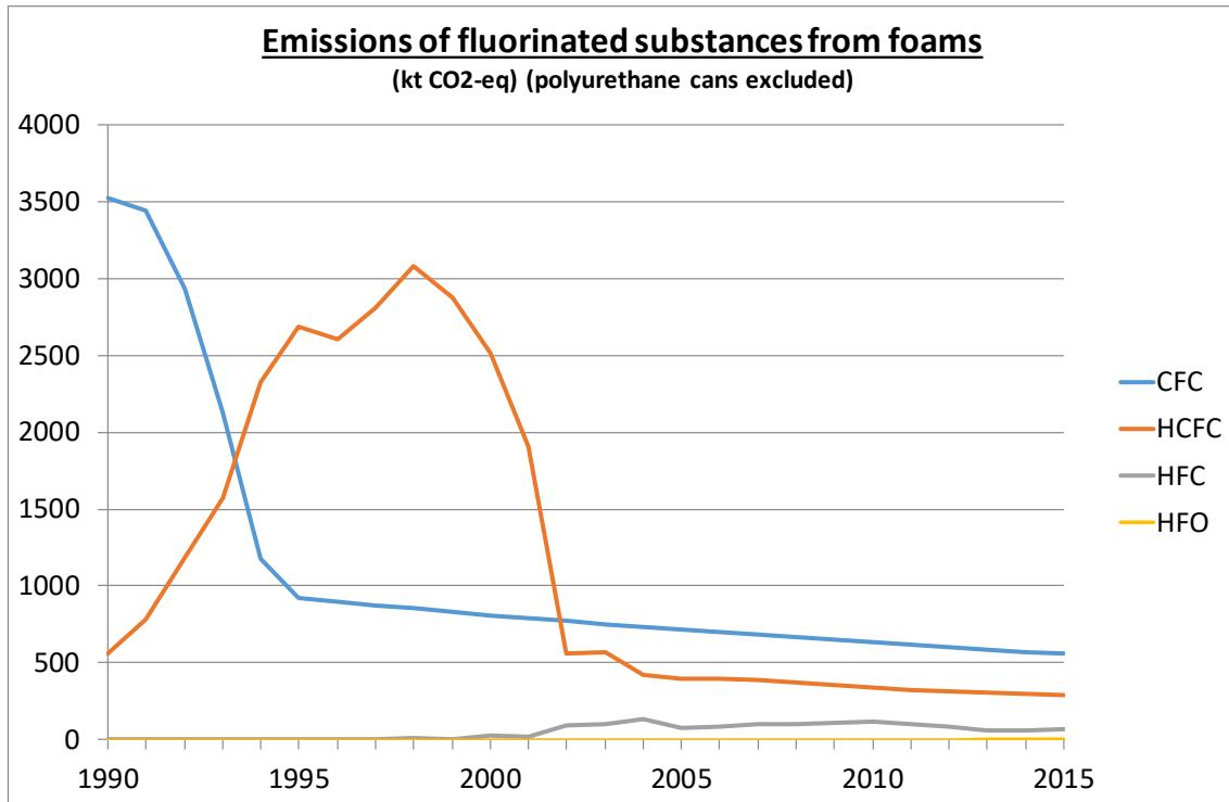
Figure 21: Emissions of F-gases from foams (kt CO<sub>2</sub>-eq)
