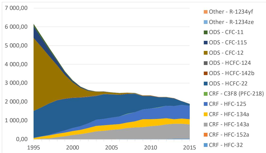
Figure 7: Emissions from refrigeration installations, by substance (kt CO<sub>2</sub>-eq)
