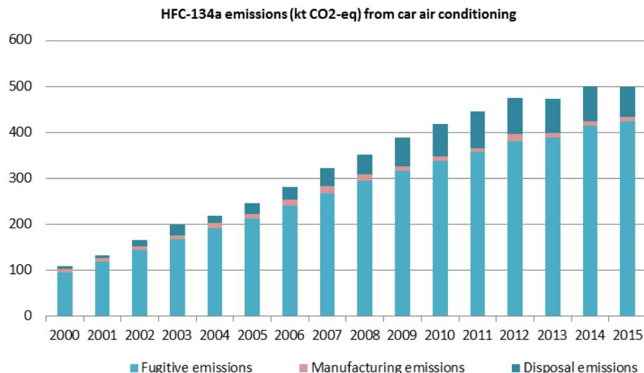
Figure 13: Emissions from car air conditioning (in kt CO<sub>2</sub>-eq)
