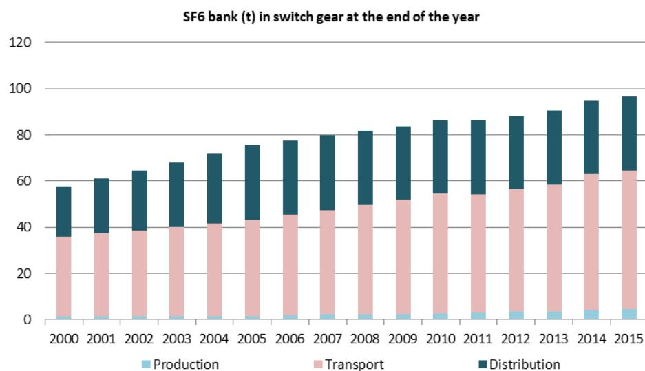
Figure 30. SF6 bank (in t) in switchgear in Belgium at the end of the year.
