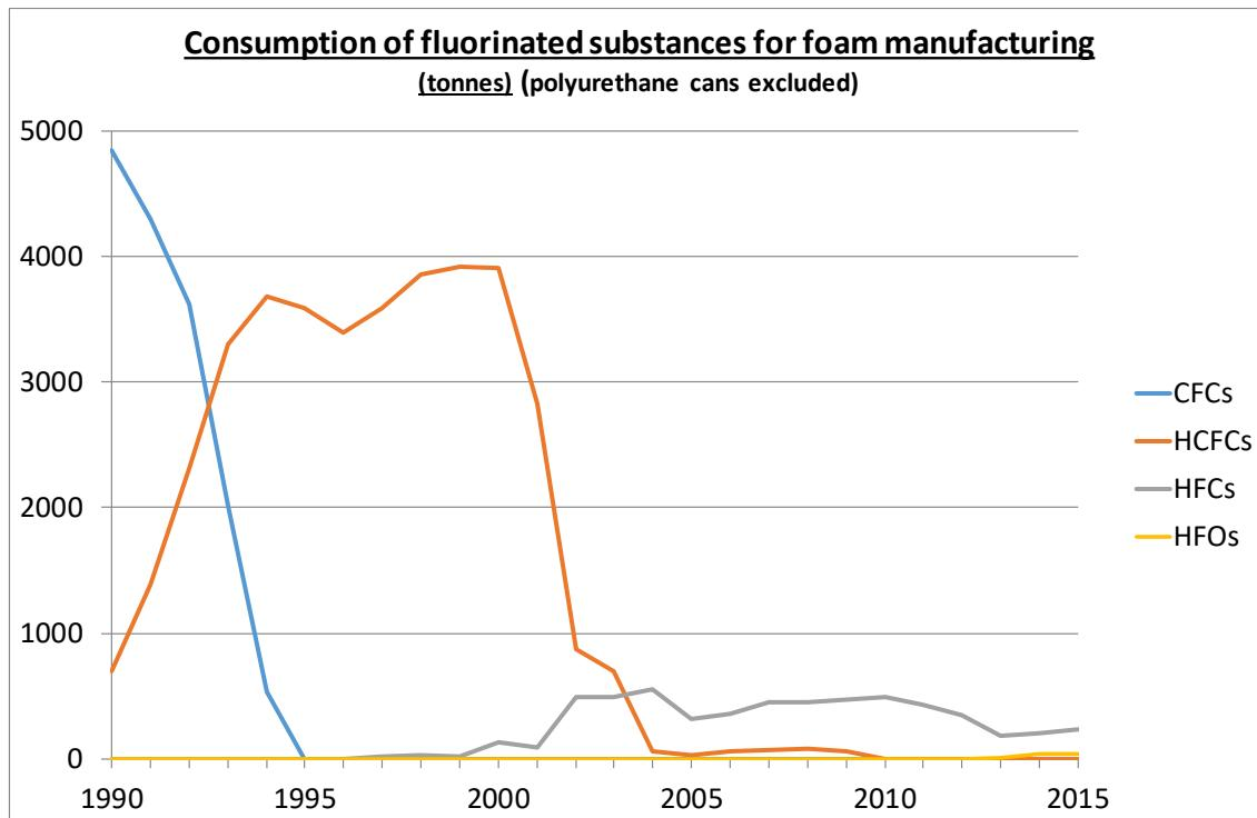
Figure 20: Consumption of F-gases for foam manufacturing (t)
